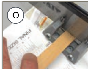
1500 Standard O. Hold bar in place and gently cut off excess. Bar should sit in slot in the middle of the clamp.
