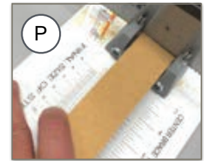
1500 Pro P. Hold bar in place and cut off excess. Pinch bar against one side of the clamp to prevent any movement during sawing.
