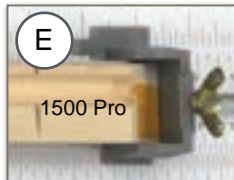
E. Make sure ends of bar is flushed against the stop
